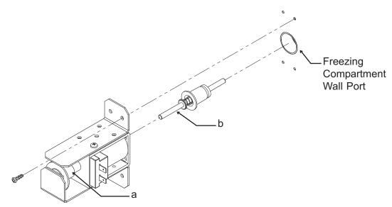
The new Harvest Assist Solenoids are interchangeable will the prior version. The b rod assembly mounts in the freezing compartment port, and the a coil assembly slips over it and attaches to the wall the same way as the prior type. These are the **new part numbers** for the service kits:
